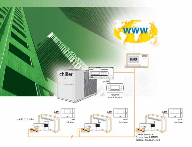
Usually, the management of large buildings (banks, office buildings, shopping centres) is centralised using a BMS that controls the lighting, security, heating and air-conditioning systems.
