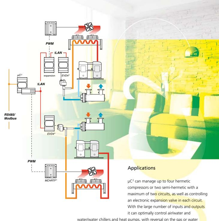
water/water chillers and heat pumps, with reversal on the gas or water circuit, air- and water-cooled units with and without reverse cycle, air/air, direct cycle and heat pump units.
