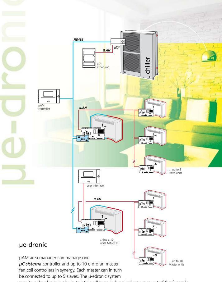
monitors the alarms in the installation, allows synchronised management of the fan coils, and implements energy-saving strategies according to the measured load and the temperature and humidity in the room.
