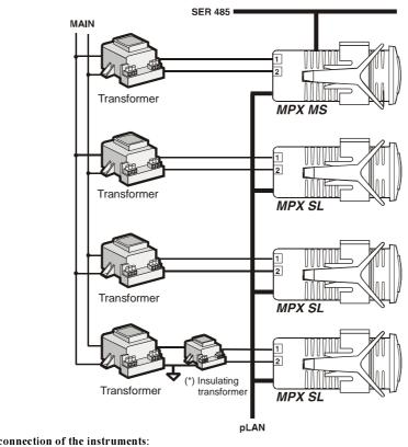
Example of wiring for serial connection of the instruments: Main = mains power supply TRF = transformer INS TRF = insulating transformer  $\overrightarrow{}$  = earth SER = multiple connection to the controller system
