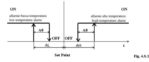
Selects the low temperature alarm. The value of AL does not indicate the alarm temperature but rather the maximum difference allowed below the Set Point.
