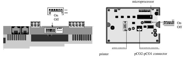
To read the address of a pCO2 board, external terminal or driver without remembering the binary code by heart, follow this simple rule: if the switch is in position 1, add up value 1 for switch 1, 2 for switch 2, 4 for switch 3, 8 for switch 4, and so on. Do not add up any values for the switches in position 0. In the example below, the selected address is: 1 + 2 + 4 + 8 = 15.
