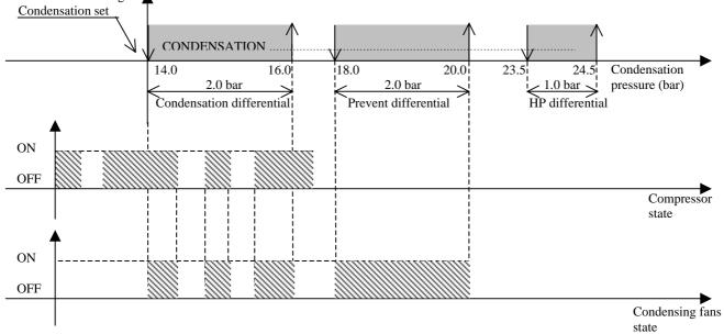
The following diagram shows fans operation with modulating outputs:
