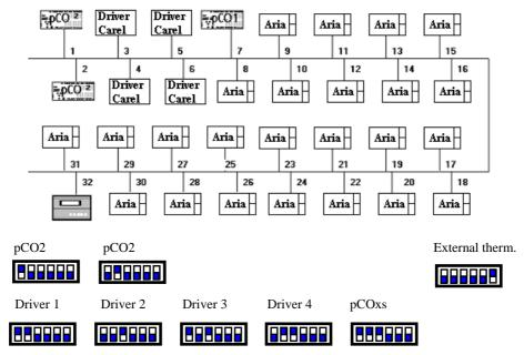
The terminals Menu main screen displays the address of the connected board in the upper right corner. Terminal add. 32 allows controlling all boards without requiring other terminals or in addition to the other terminals; the program allows terminal with add. 32 to access the parameters of all connected boards, one by one. Passage among the boards can be executed by simply pushing button info.
