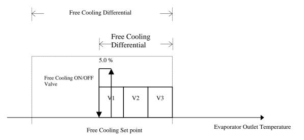
Here is an example of Free Cooling control with ON/OFF valve and three condensation steps.
