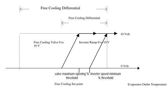
The devices, whether they are valve or fans, will be activated in the second half of the control differential through the effect of the integrating control. Their activation will be tied to the set integrating constant: the slower it is, the greater the value attributed to the specific parameter.
