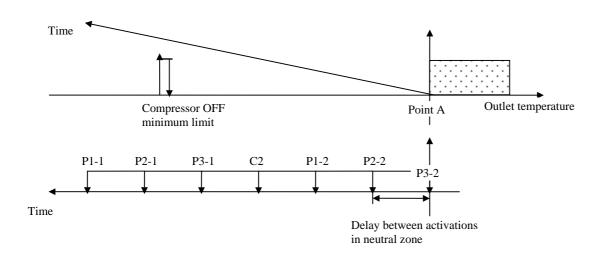
As long as the temperature is lower at point A, the compressors are activated with a delay between activations equal to parameter "delay between power-downs in neutral zone":
