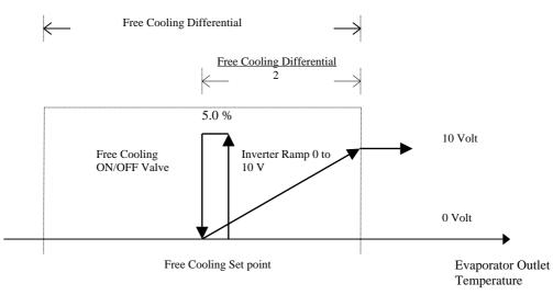
The devices, whether they are valve or fans, will be activated in the second half of the control differential through the effect of the integrating control. Their activation will be tied to the set integrating constant: the slower it is, the greater the value attributed to the specific parameter. The amplitude of the valve control step will be 5.50% of the said control differential. All proportional outputs relating to the different units of the system will be piloted in parallel
