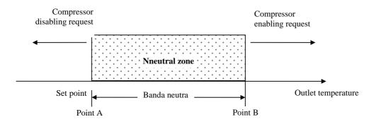
As long as the temperature remains inside the neutral zone, no compressor is enabled or disabled (outlet temperature between point A and point B). Compressor enabling request (outlet temperature higher at point B):
