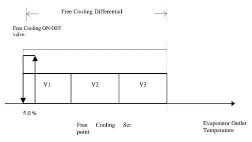
Here is an example of Free Cooling control with ON/OFF valve and three condensation steps.
