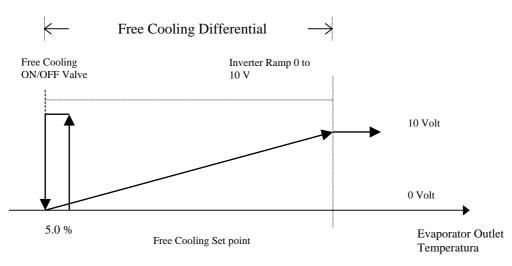
The ON/OFF valve activation step will, in any case, be positioned in the first part of the control differential and will have an amplitude of 5.0% of the said differential.
