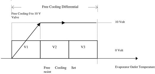
The proportional control ramp of the Free Cooling valve will be calculated inside the first activation step of the condensation fans. In this way, when the first fan is enabled, the valve will be completely open, and, therefore, water flow in the Free Cooling exchanger will be at maximum level.
