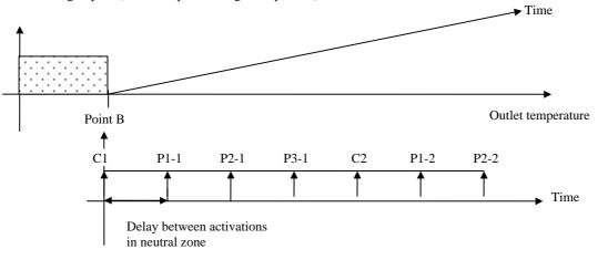
As long as the temperature is higher at point B, the compressors are activated with a delay between activations equal to parameter "delay between activations in neutral zone": Disabling active devices:
