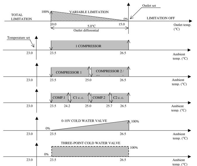
As shown in the diagram, if outlet temperature ranges between outlet set point and outlet differential, the cooling devices are limited only partially; the more temperature decreases the more limitation increases.
