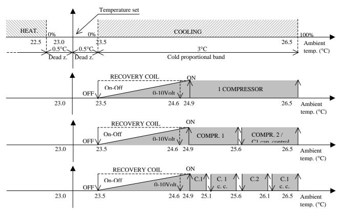
11.3 **RECOVERY WITH COOLING DEVICES ON CLOSE CONTROL UNITS WITH WATER COILS** The following diagram shows how the cold coil steps are offset compared to normal position to ensure energy saving.
