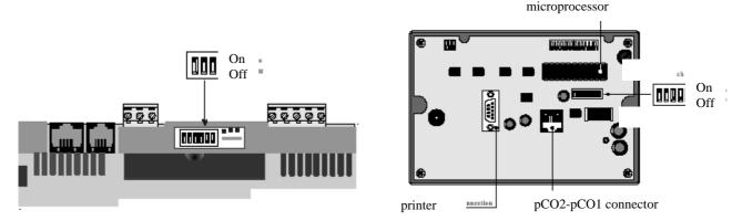
To read the address of a pCO2 board, external terminal or driver without remembering the binary code by heart, follow this simple rule: if the switch is in position 1, add up value 1 for switch 1, 2 for switch 2, 4 for switch 3, 8 for switch 4, and so on. Do not add up any values for the switches in position 0. In the example below, the selected address is: 1 + 2 + 4 + 8 = 15.
