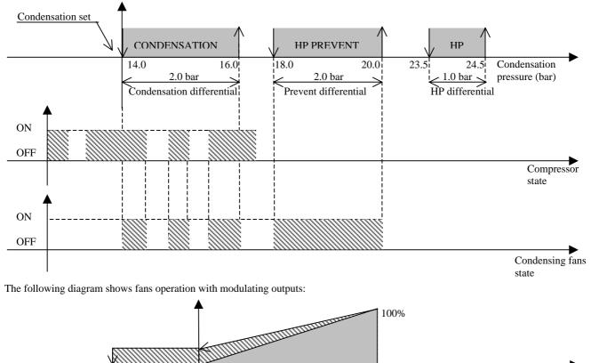
Condensation differential Opening start point (100%) Opening end point (0%)
