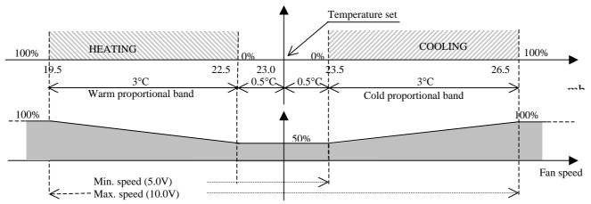
During dehumidification, speed is automatically decreased to 5.0V (50%) default value, modifiable if required. The minimum and maximum speeds default values correspond to 5.0V and 10.0V, modifiable if required.
