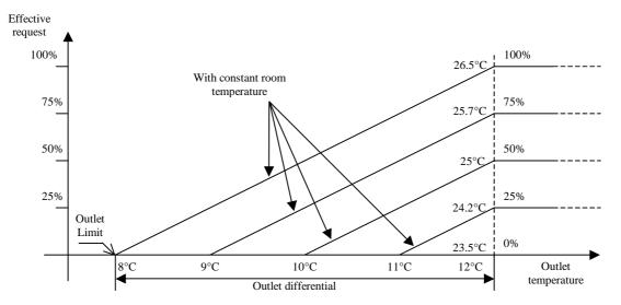
As can be seen, if the outlet temperature is between the outlet set point and the outlet differential, the cooling devices are increasingly limited as the temperature lowers.
