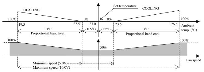
The minimum and maximum speed of the fan can be set. The default values 5.0V and 10.0V.
