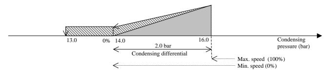
The maximum and minimum speed of the condenser fans can be set; if the minimum speed set is greater than 0V, the fan will be able to operate at the minimum speed down to 1.0 bar below the condensing pressure set point before stopping altogether (see the dashed part in the graph above).
