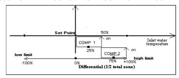
Note: the example above refers to cooling applications (Summer mode). For heating applications (Winter mode), the steps will be positioned specularly with respect to the set-point.
