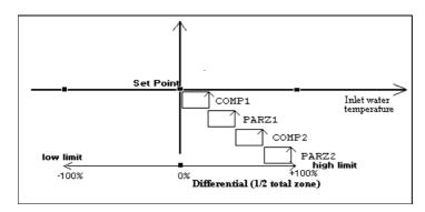
Note: the example above refers to cooling applications (Summer mode). For heating applications (Winter mode), the steps will be positioned specularly with respect to the set-point.
