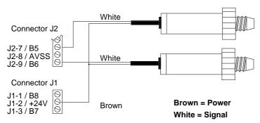
Connect the transducers directly to the interface
