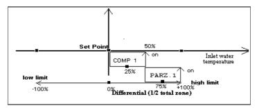
Note: the example above refers to cooling applications ('Summer' functioning mode). For heating applications ('Winter' functioning mode), the steps will be positioned specularly with respect to the set-point.
