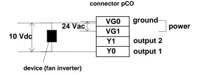
The figure above shows pCO's analogue outputs connections. Power terminals VG0 and VG1 by 24 Vac.
