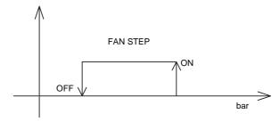
During the defrosting cycle the fans relative to the circuit undergoing such a procedure will be forced into the OFF status.
