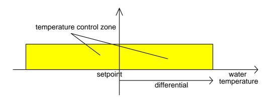
In the application shown in the figure above the set-point has been set so as to represent the **CENTRAL** point of the regulation zone.
