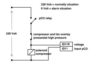
When pCO's relay enabling the compressor's functioning is closed and that relative to the high pressure pressurestat is open, the 'high pressur alarm' will be detected through the 220 Volt input.
