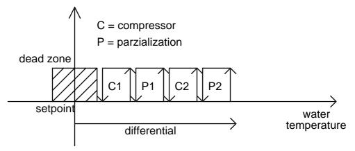
Note: the range of the dead zone must be inferior to the selected differential otherwise the connected devices will not activate.
