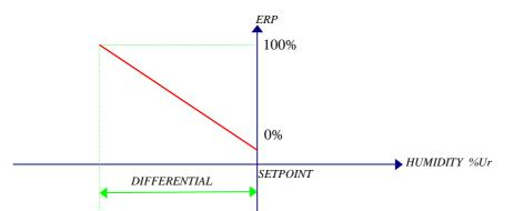
The humidifier regulation graph depends on the nominal Output, set Output and ERP proportional error:
