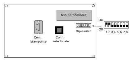
Each switch is numbered from 1 to 6, and the addressing must be carried out beginning from the switch number 1; below a certain number of addressing examples are given.
