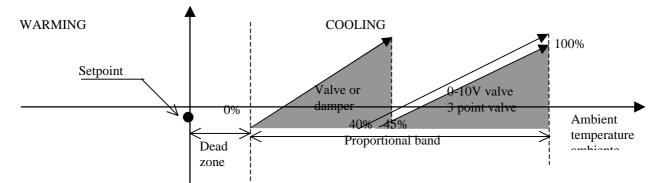
The range of the two valves in free cooling is reduced from 40% of the proportional band to 100%. As in the other cases, the free cooling valve or damper modulates up to 45% of the proportional band and this allows a slight overlap of the valves.
