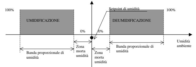
The Proportional band and Dead zone, selectable from mask, are automatically applied both on the humidification zone and on the dehumidification zone. When the dead zone is 0, the proportional band starts in proximity to the setpoint and consequently turns out to be shifted with respect to the graph.
