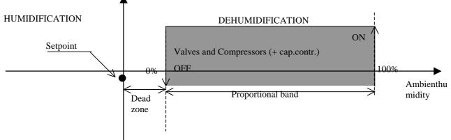
All the activated humidification devices follow the behaviour of the step being displayed, with the consequent occupation of the whole proportional band. Actually, the start and stop values are as follows:
