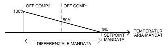
As you can see in the graph, the limiting action increases proportionally to reduction of the temperature below the supply setpoint. It reaches its maximum when it is equal or less than:
