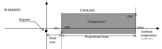
The choice of only one compressor involves the occupation of the whole proportional band, in fact the On and Off values are as follows: ON COMP.  $\rightarrow$  Ambient temperature > (Setpoint + Dead zone + Proportional band) OFF COMP.  $\rightarrow$  Ambient temperature < (Setpoint + Dead zone)
