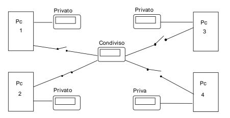
In this example the shared terminal is associated to 4 pCO2 cards but only the card with addr. 2 can be visualised and can receive the keypad commands from it. The switching between the cards occurs, cyclically  $(1\rightarrow 2\rightarrow 3\rightarrow 4\rightarrow 1...)$ , by pressing the *info* button. The switching can also take place automatically on direct request by the program.
