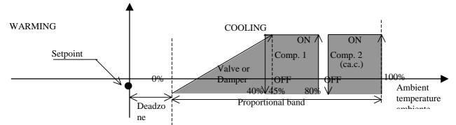
In this case the two steps equally share the zone of proportional band from 40% to 100%. The Carel manufacturer's values schedule two identical steps as shown in the graph. The free cooling valve or damper modulates from 0% to 45% of the proportional band.
