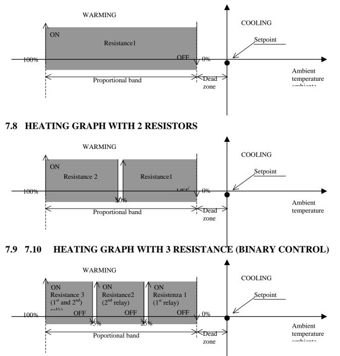
By binary management is meant a control of a number of resistors higher than the available outputs, applying the binary logic. The use of this system involves an electronic device connected to two outputs, being able to read the code and consequently activate the resistance.
