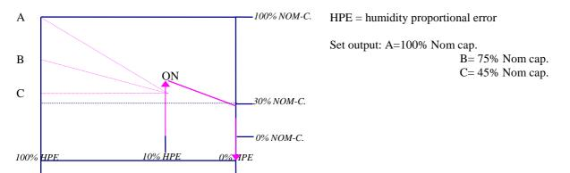
The humidifier has a minimum output of 30% of the Nominal power (for technical reasons) when ERP = 0% and it increases as the ERP increases until the output being set with ERP=100% is reached. The humidifier is managed so as not to be started with minimum values of ERP, otherwise the minimum output, 30% Nom. capacity, would cause an excessive humidity increase. To face this drawback, the humidifier starts obviate when the ERP value is at least 10%.
