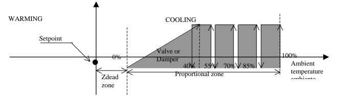
In this case the four steps share equally the proportional band zone ranging from 40% to 100%. The Carel manufacturer's values schedule four identical steps as shown by the graph. The free cooling valve or damper modulates from 0% to 45% of the proportional band.
