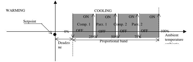
The four step selection (2 compressors with capacity control) involves the occupation of the entire proportional band exactly divided into four halves; actually, the On and Off values are as follows :
