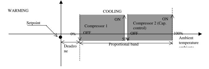
The two step selection (2 compressors or 1 compressor with the capacity control) involves the occupation of the entire proportional band exactly divided into two halves; actually, the On and Off values are as follows : ON COMP.1  $\rightarrow$  Ambient temperature > (Setpoint + Dead zone + 50% Prop.band) OFF COMP.1  $\rightarrow$  Ambient temperature < (Setpoint + Dead zone)
