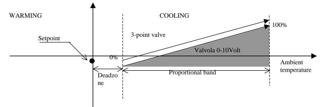
As you can see, the characteristic of the two valves is the same and actually the effect is the same, namely they are open from minimum (0%) to maximum (100%) proportionally to the proportional band. The difference between the two valves is only due to the type of driving that in one case is a 0-10V modulating signal, more precise, whereas in the other case the management is provided by 2 time-activated relays, and is less precise.
