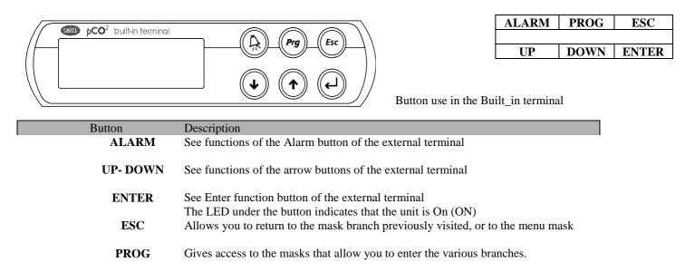
The Built-in terminal, lacking the ON/OFF button, carries out the switching on and off of the unit (On-Off) positioning itself on the main mask and pressing the arrow upwards this mask will be displayed where it is possible to start and stop the unit.
