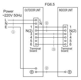
Note: 1) Power cable 3X2.5mm<sup>2</sup> ②Intercnnecting cable 3X1.0mm<sup>2</sup> ③Signal core 3X0.75mm<sup>2</sup>
