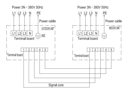
Electrical wiring diagram of the cooling only models
