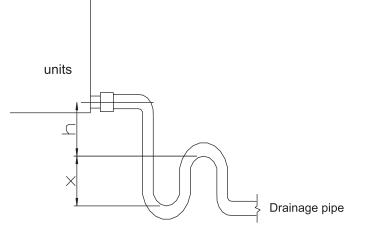
Drainage pipe connection drawing
