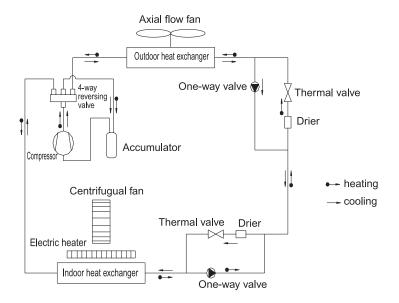
Working elements diagram of heat pump unit(Using expansion valve)
