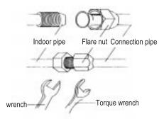
4. When there is a connector between pipes, it should be fixed tightly, if indoor and outdoor unit is close enough to use one connection, it is better to use one.
