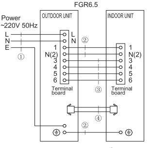
Note:①Power cable 3X4mm<sup>2</sup> ②Intercnnecting cable 3X2.5mm<sup>2</sup> ③Signal core 4X0.75mm<sup>2</sup> ④Signal core 2X0.75mm<sup>2</sup>
