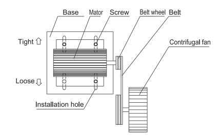
The tightness level of belt is tested by tension meter as shown below, when ?reaches the deviation length (deviation length=--),read the value on the meter, the value should be in the category specified in the sheet.
