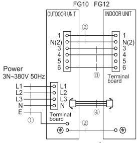
Note:①Power cable 5X1.5mm<sup>2</sup> ②Intercnnecting cable 3X1.0mm<sup>2</sup> ③Signal core 3X0.75mm<sup>2</sup> ④Signal core 3X0.75mm<sup>2</sup>
