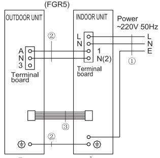
Note: Dewer cable 3X2.5mm<sup>2</sup> 2 Intercnnecting cable 3X2.5mm<sup>2</sup> 3 Signal core 6X0.75mm<sup>2</sup>
