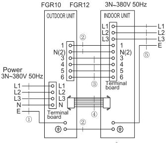
Note: ①Power cable 5X1.5mm<sup>2</sup> ②Intercnnecting cable 3X1.0mm<sup>2</sup> ③Signal core 4X0.75mm<sup>2</sup> ④Signal core 6X0.75mm<sup>2</sup> ⑤Power cable 4X1.5mm<sup>2</sup>
