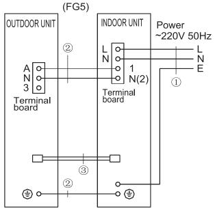
Note: Dewer cable 3X2.5mm<sup>2</sup> 20 Intercnnecting cable 3X2.5mm<sup>2</sup> 30 Signal core 2X0.75mm<sup>2</sup>
