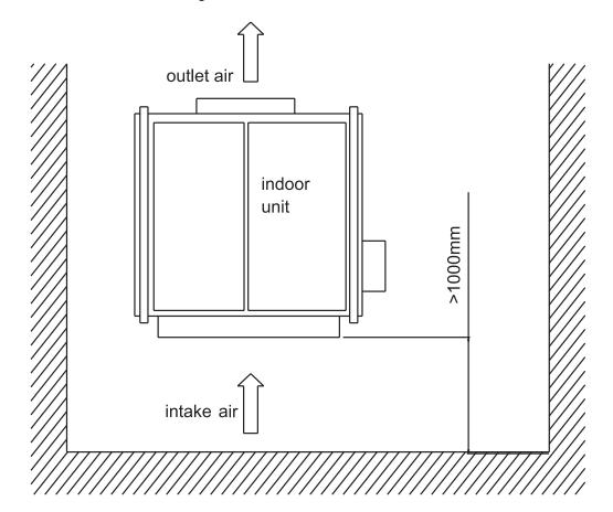
Figure 2 for indoor unit installation
