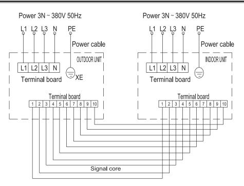
Electrical wiring diagram of the heat pump units
