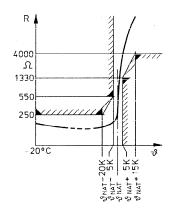
Fig. 6: Thermistor Resistance Curve
