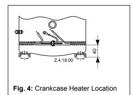
The crankcase heater must be mounted below the oil removal valve located on the bottom shell. The crankcase heater must remain energized during compressor off cycles.
