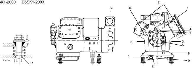
Note: The D6SK can be mounted to fit a 6-cylinder or 8-cylinder footprint. (See page 7- Mounting Parts)
