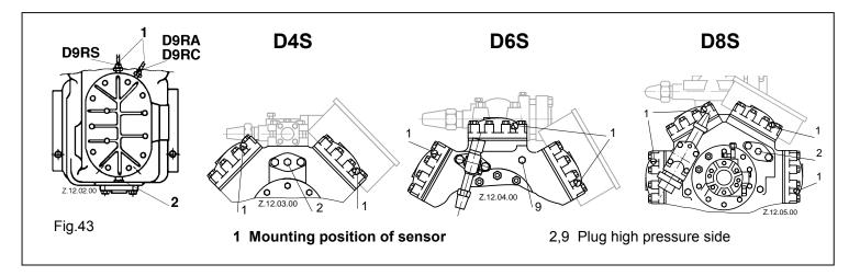
With the standard compressor D9R, there are no holes for the discharge temperature protection, therefore the cylinder head has to be changed for the subsequent sensor installation.
