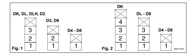
Fig. 1: stacking height for transport
