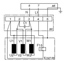
Fig.19 Steinmetz Connection for Single-phase operation
