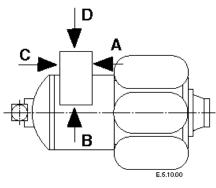
Standard terminal box with enclosure class according IEC 34: IP 54
