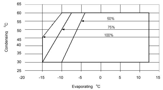
**Diagram 5** Suction gas temperature 25<sup>°</sup>C
