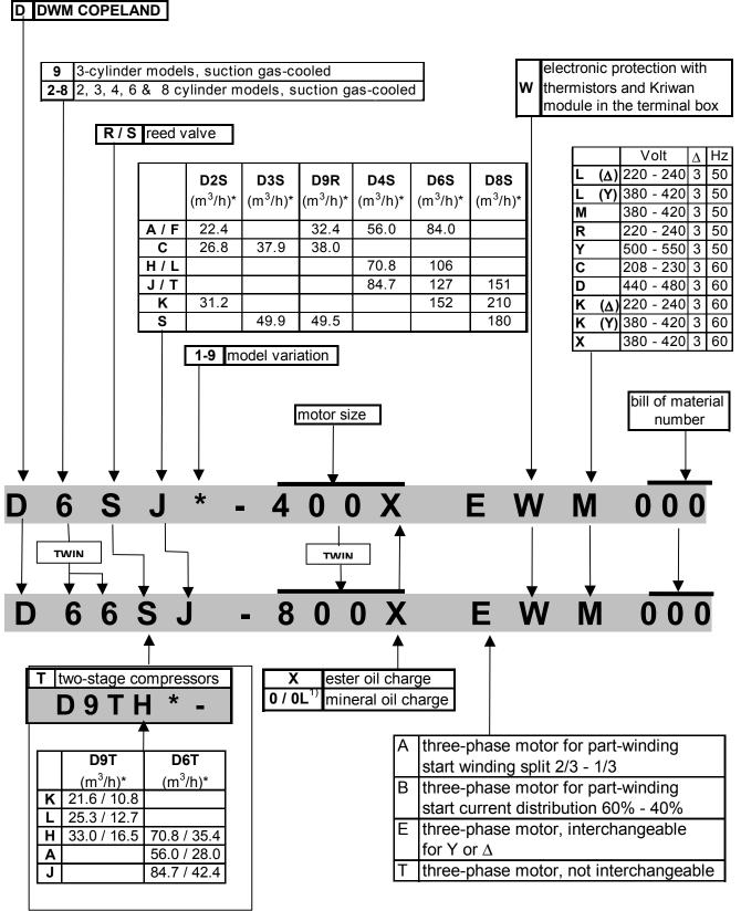
• Displacement at 1450 min<sup>-1</sup>, 50Hz;
