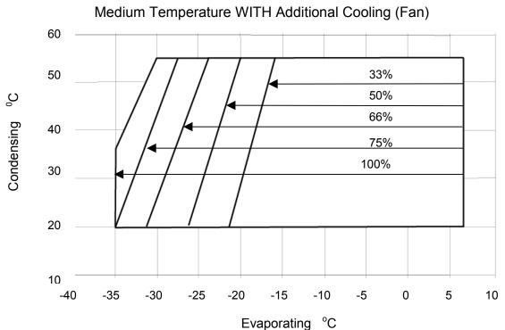
**Diagram 9** Suction gas temperature 25<sup>o</sup>C
