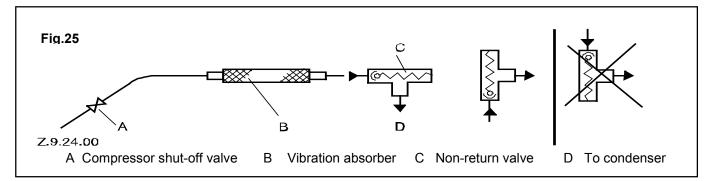
A non-return valve must be installed in the discharge line to prevent the refrigerant from flowing back from the condenser to the suction side using the by-pass line.
